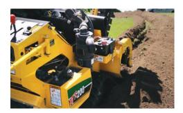
SLENDER PROFILE. The 35" (88.9 cm) width allows the RTX200 to access compact spaces including passing through typical backyard gates.
