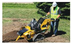
**ENHANCED VZ STEERING.** Operators can steer the machine using only the handlebars — rather than traditional methods using levers or steering wheels. These bars also provide additional leverage when operating on difficult terrain.
